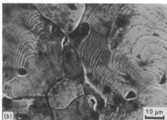
Figure 10a and b Surface appearances of a siliconized sample after 6 min of CVD treatment at 1000 °C (total gas flow rate: 1.85 h -1 ; Ar 21 vol%; SiH 4 0.6 vol%; SiCl 4 20 vol%; H 2 58.4 vol %).
